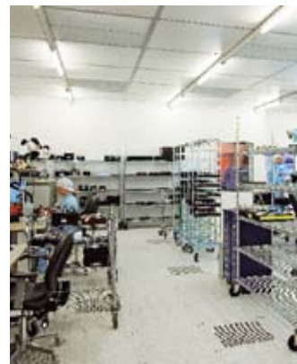
In the clean room all the air is changed out 55 times per hour. Here it is always 21°C with a relative humidity of 45%.
